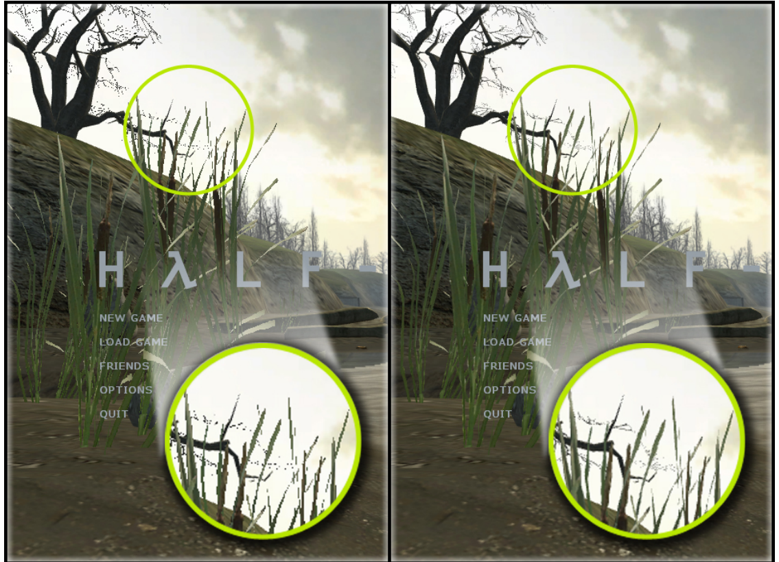
Figure 14. Normal Antialiasing (Left) vs. Transparent Adaptive Antialiasing with Clear, Realistic, Small Branches and Foliage (Right)
